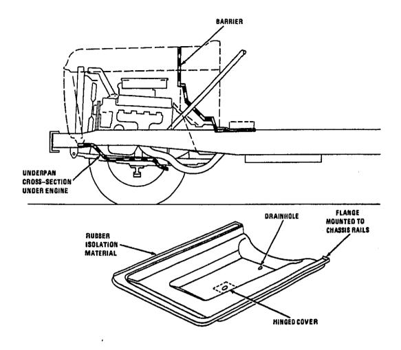
FIGURE 5-10. Possible Underpan Configuration
