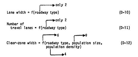
Lane widths are 15 feet for interstate roadways and 12 feet for all other roadways. The number of travel lanes is two for all local roadways and four for all other roadways. The clear-zone widths are more complicated functions, as indicated in equation D-12. The clear-zone widths used in the model appear in Table D-13. The definition of the clear-zone distance is based upon the best information currently available (References 44, 46, 59).
